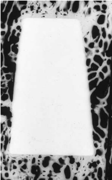
26.6 Contact micro-radiograph of the AW-GC vertebral prosthesis which bonded to the bone trabeculae of vertebral bodies of sheep (6 months after implantation).
