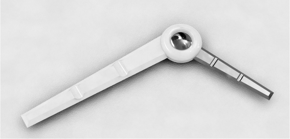
Fig. 4.4 To reduce rigidity, polyethylene (PE) was soon introduced in the articulation mechanism and it often replaced at least one stem, as shown in this scheme which resembles the St George Bucholtz (early design) with a fitting metal–polyethylene hinge
