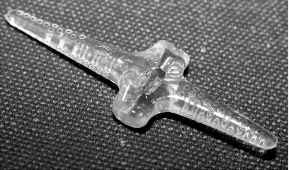
Fig. 4.8 An ex vivo retrieval of a Swanson prosthesis in which very little superficial wear can be seen, despite its 12 years in service in vivo
