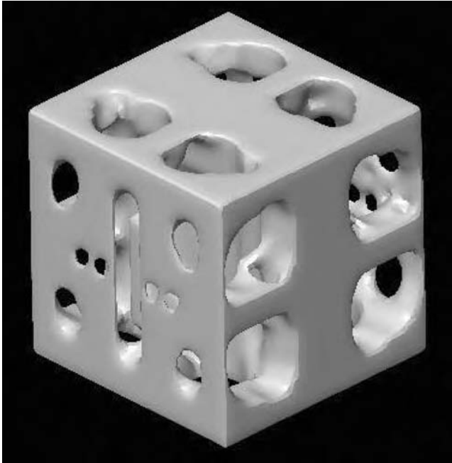
Figure 7.4 Example of unit cell designed using full microstructure topology optimization methods. This cell is repeated in 3D space to create the complete scaffold architecture.
