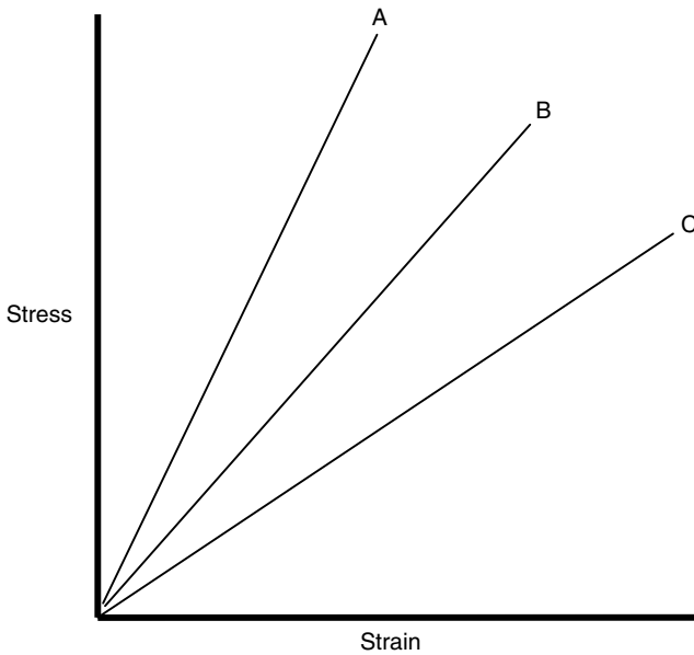
Figure 10.9 The mechanical properties of a rate-dependent biological material vary with the rate of load application. Higher rates of load application (A) cause a stiffer response to an identical load in an intermediate rate (B) and a slow rate of load application (C).
