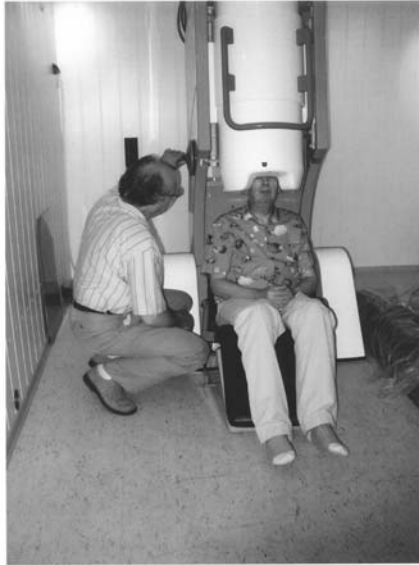
Figure 4.5 Patient being treated for Parkinson's disease by Dr. Photios Anninos. Dr. Anninos is shown adjusting a liquid helium cooled Superconducting Quantum Interference Device to obtain magnetoencephalogram data. (Courtesy of Dr. Photios Anninos, University of Thrace, Department of Medicine, Medical Physics Sector, Alexandroupolis, Greece. Permission given by IABC Foundation.)
