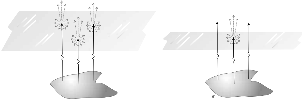
Figure 5-3 Thick crystals stop a larger fraction of the photons.
