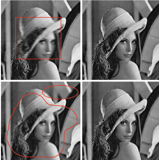
■ Fig. 25-23 Non-blind space-variant restoration. Left column: spatially variant motion blurred images. Right column: the corresponding recovered images using the suggested method
