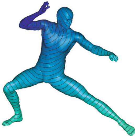
■ Fig. 32-4 Distance map measured on a curved surface. Equi-distant contours from the source located at the right hand are shown. Reproduced from [25]
