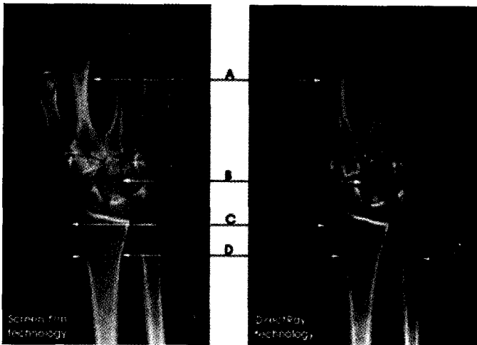
Fig. 3.38. Comparison of radiographies of the same human hand taken at equal dose with screen-film technology ( left ) and Direct Radiography Corp.'s DirectRay® technology ( right ), compared specifically in four points indicated by the arrows, may reveal the comparable or better overall image quality of this a-Se based detector [50].
