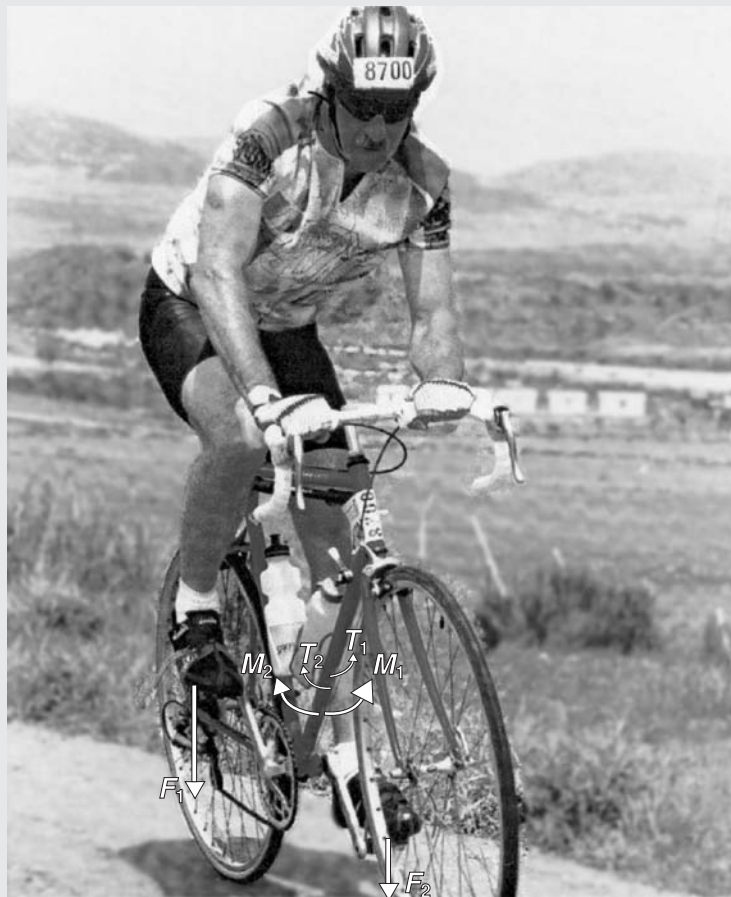
Fig. E1.1 Bending moments ( M_1 and M_2 ) and torsional torques ( T_1 and T_2 ) generated in bicycle frame by forces F_1 and F_2 applied to pedals.
