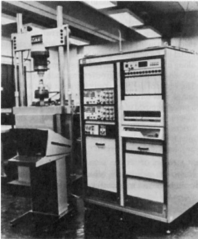
Fig. 3.2 A servohydraulic universal testing machine linked to a computer. (Courtesy of MTS Systems Corp.)
