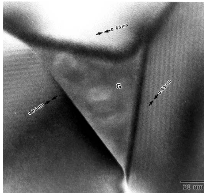
Fig. 5.36 Glassy phase at triple point in silicon nitride; notice the individual crystallographic planes in \text{Si}_3\text{N}_4 . (Courtesy of K. S. Vecchio.)
