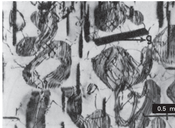
Fig. 10.16 Interfacial dislocations formed in a semicoherent precipitate. (From G. C. Weatherly and R. B. Nicholson, Phil. Mag. , 17 (1968), 801.)
