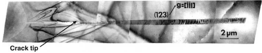
Fig. 7.9 Dislocations emitted from a crack tip in copper. (Courtesy of S. M. Ohr.)
