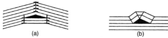
Fig. 8.5 Crack nucleation by (a) lattice rotation due to bend planes and (b) deformation twins. (c) Crack nucleation in zinc due to lattice rotation associated with bend planes. (Reprinted with permission from J. J. Gilman, Physical Nature of Plastic Flow and Fracture , General Electric Report No. 60-RL-2410M, April, 1960, p. 83.)
