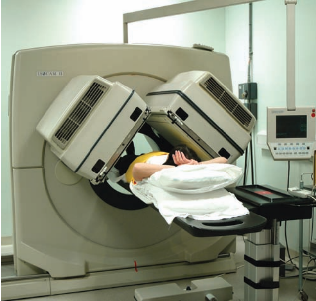
Figure 2.5 A dual-head general purpose gamma camera with the detectors in a 90° configuration for cardiac imaging. An example of a dedicated cardiac imaging system can be seen in Figure 1.1b.
