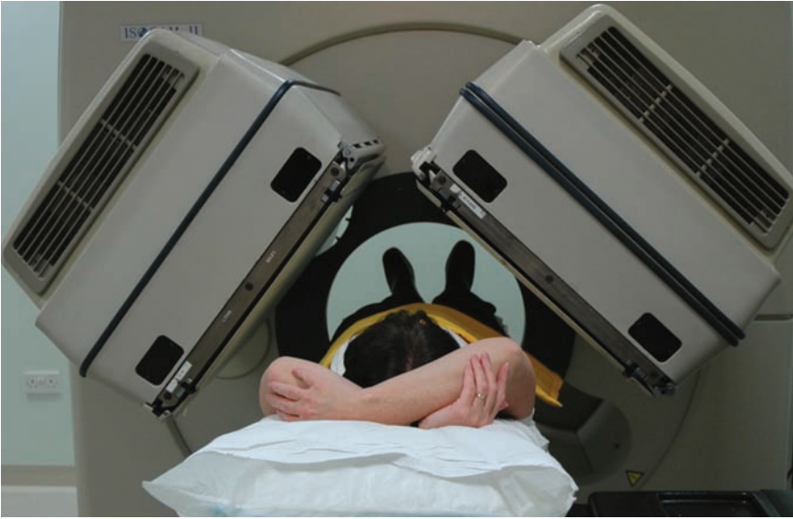
Figure 5.5 Large field of view (LFOV) dual-head gamma camera with the detectors moving to a 90^\circ configuration for cardiac imaging.
