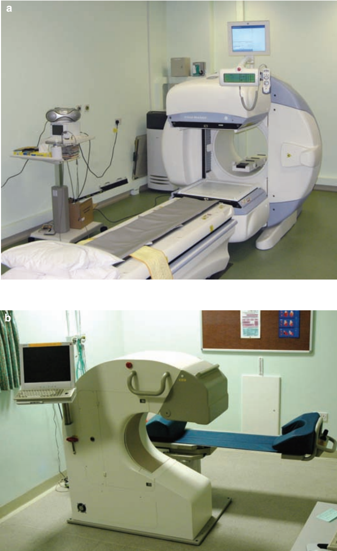
Figure 1.1 (a) Double-headed general purpose gamma camera. Each head contains a large, flat crystal of sodium iodide, which emits visible light when it absorbs a gamma ray photon. The resulting pattern of light flashes is detected and converted into a digital electronic image by a bank of photomultiplier tubes mounted on the back of the crystal. The heads rotate around the patient and acquire data from a volume which includes the heart. These data are stored in a dedicated computer and processed to produce a series of slices through the left ventricle (Figure 1.3). This particular model incorporates a low-dose computed tomography (CT) scanner in the gantry, allowing the acquisition of scintigraphic and CT images without moving the patient. These images can be superimposed, providing precise anatomical location of scintigraphic abnormalities. In nuclear cardiology practice, the CT data can be used to correct the MPS images for attenuation effects. However, this is not currently part of our routine practice. (b) Smaller footprint camera used in our nuclear cardiology department.
