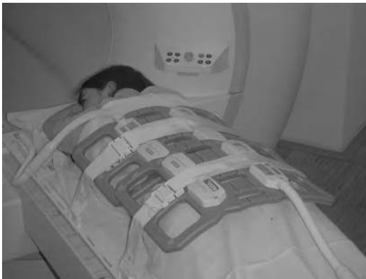
FIGURE 1 A combination of two phased-array coils is used for MRC. Thus, coverage of the entire colon in conjunction with homogenous signal reception is guaranteed.
