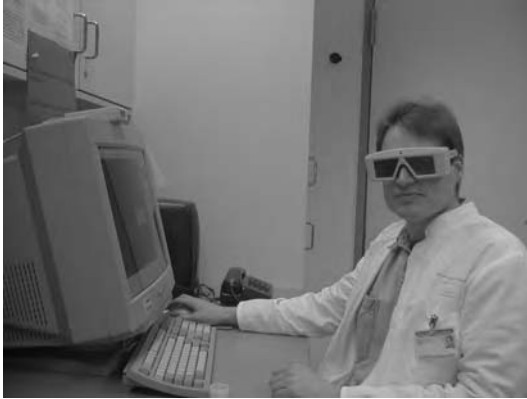
FIGURE 13 A three-dimensional plastic effect can be produced at the workstation by using a special software and shutter-glasses (stereo viewing).
