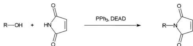
Figure 32.14 Mitsunobu alkylation of maleimide with alcohols (method 3).
