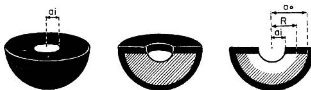
Figure 43.7 Cross section of hemisphere-shaped matrix coated with an impermeable layer of polymer that restricts the release of drug to the aperture. Release rates are predicted to be constant when R \gg a_i hr. (Reprinted with permission from Harcourt Academic Press.)
