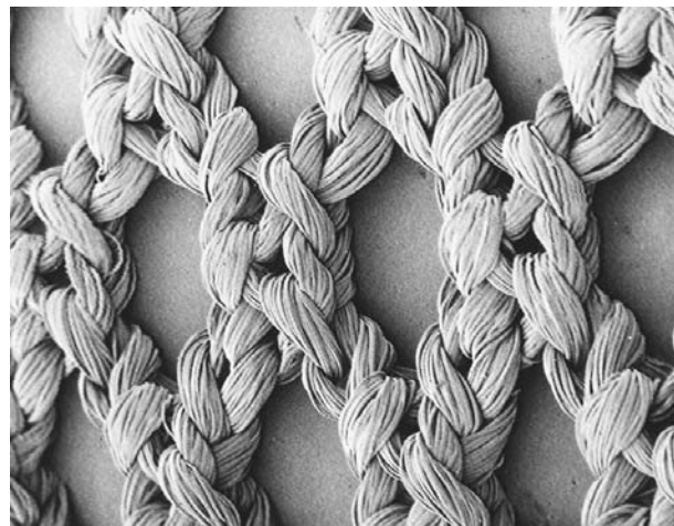
Figure 19.11 Scanning electron micrograph of PTFE mesh at 22 \times . (From C. C. Chu, B. Pourderyhm, and L. Welch. Characterization of morphologic and mechanical properties of surgical mesh fabrics. J. Biomed. Mater. Res. 19:903–916 (1985).)
