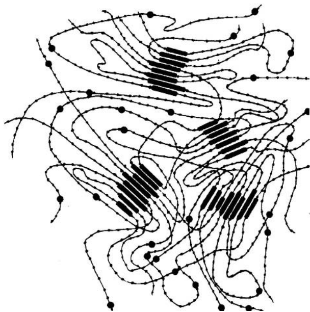
Figure 13.9 Distribution of hard and soft segments in a polyurethane elastomer. (From Ref. 63.)
