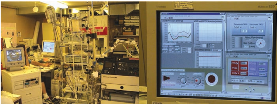
FIGURE 13 Mock loop overview including an IVUS and ICUS, pulse generator, hemodynamic measurement unit, and a computer aided flow analysis station.
