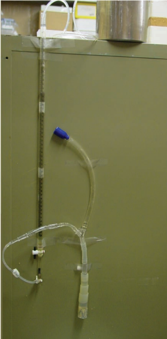
FIGURE 6 Static leakage test setup for the first-generation pulmonary devices.
