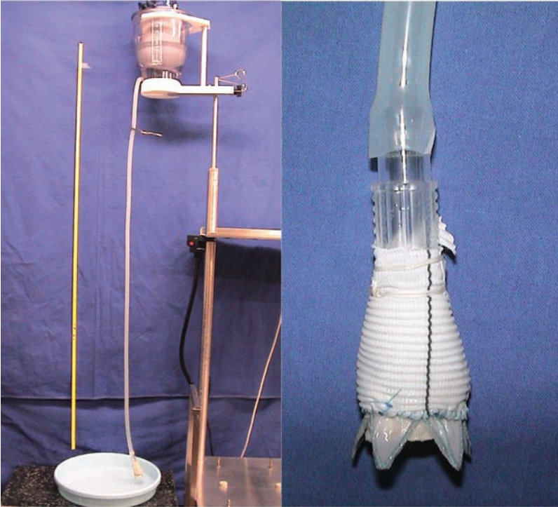
FIGURE 12 Static leakage test-column setup for the mitral device.
