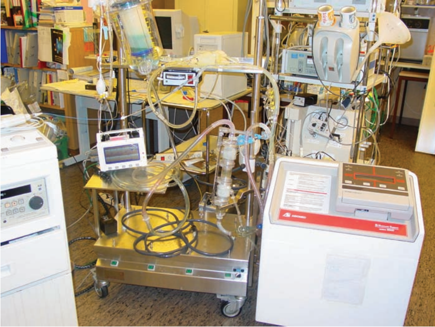
FIGURE 7 Overview of the mock loop setup for dynamic valved stent testing.
