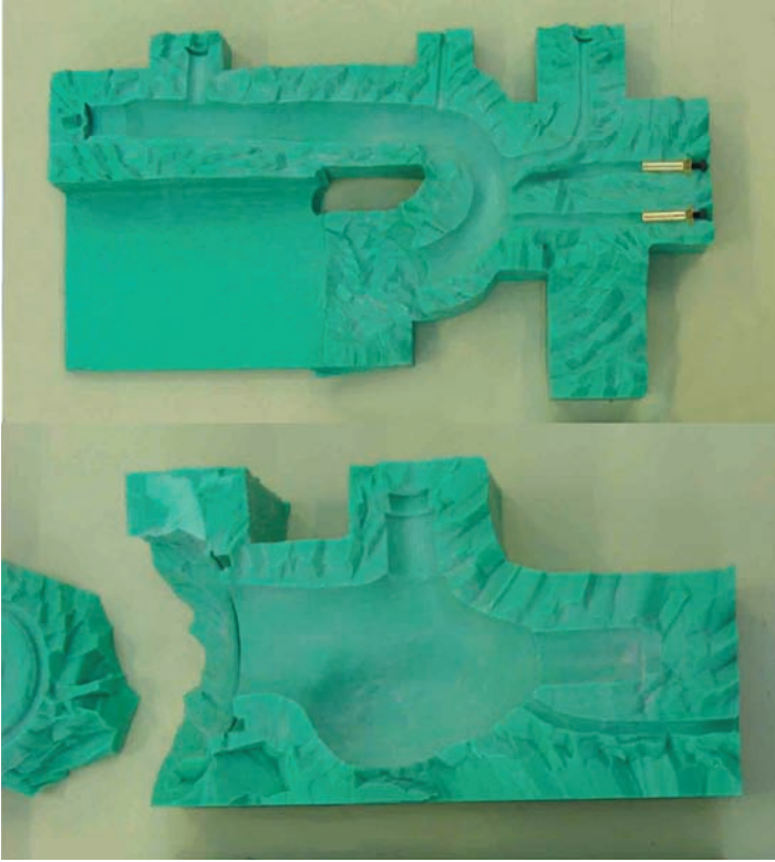
FIGURE 3 Reversed silicon master mold.
