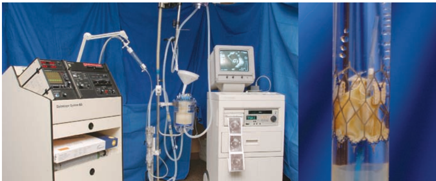
FIGURE 10 Aortic valved stent device mock loop bench test setup including a pulsatile flow generator, an expansion reservoir, a valve chamber, and an intravascular assessment unit.
