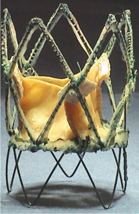
FIGURE 5 Aortic valved stent made from three linked nitinol Z-stents and a pericardial tissue valve—ready to use.
