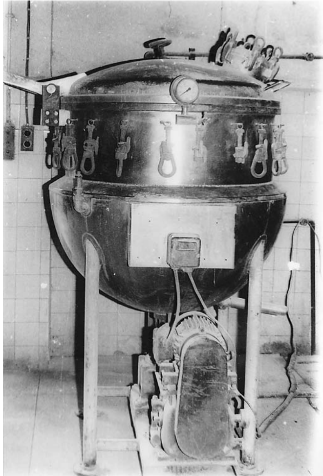
Figure 11 Holding of ogi slurry in a stainless-steel, steam-jacketed kettle at 40°C for spray-drying. (Courtesy of the Federal Institute of Industrial Research, Oshodi, Lagos, Nigeria.)
