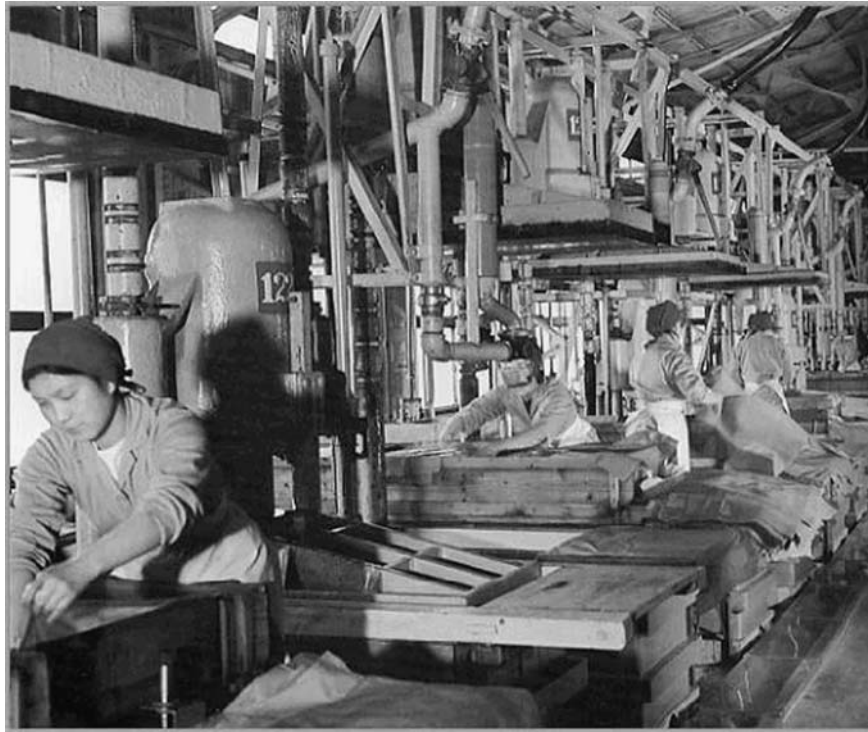
Figure 36 Box-type hydraulic machine. (Courtesy of the Kikkoman Corporation.)
