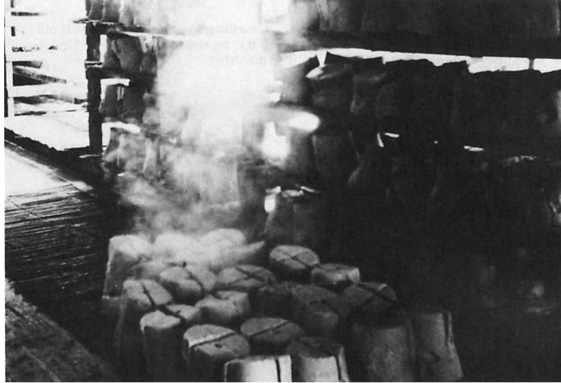
Figure 15 Cooling of cooked soybeans molded into large miso-dama for cooling. (Courtesy of Central Miso Research Institute.)
