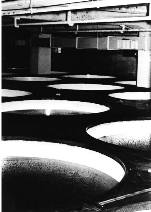
Figure 33 Iron fermentation tanks lined with epoxy resin, which was installed in 1965. (Courtesy of the Kikkoman Corporation.)
