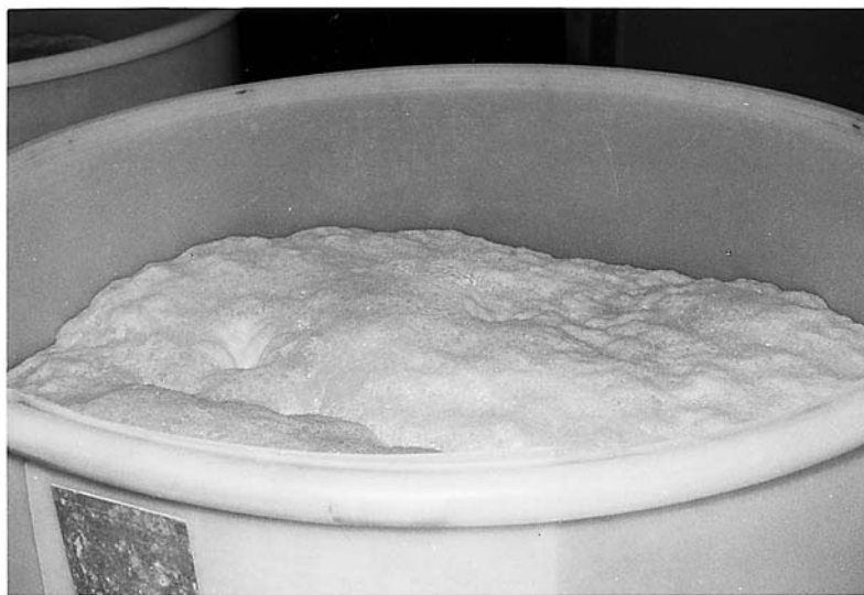
Figure 14 A large amount of foam is formed during moto and moromi mash fermentation.
