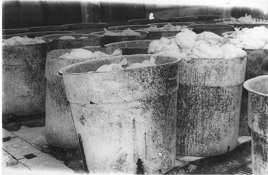
Figure 14 Commercial industrial gari production. Bagged pulped roots fermenting in plastic open-bottom modern vats. (Courtesy of the Federal Institute of Industrial Research, Oshodi, Lagos, Nigeria.)
