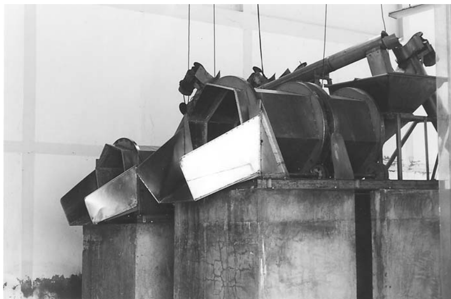
Figure 9 Mixer for fast and thorough mixing of fish and salt. (Courtesy of Pichai Fish Sauce Co., Ltd.)
