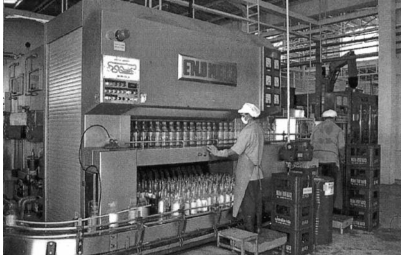
Figure 11 Bottle cleaning machine. (Courtesy of Pichai Fish Sauce Co., Ltd.)
