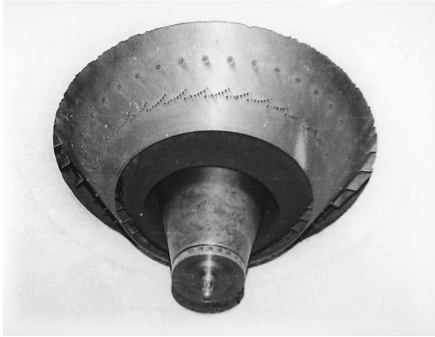
Figure 12 Drying of ogi slurry in a Niro atomizer spray-dryer showing the atomizer spray nozzle. (Courtesy of the Federal Institute of Industrial Research, Oshodi, Lagos, Nigeria.)
