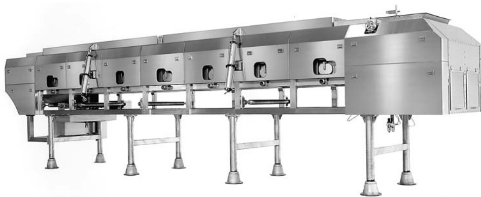
Figure 6 Steel-belt-type continuous rice steaming equipment. (Courtesy of Fujiwara Techno-art Co. Ltd.)
