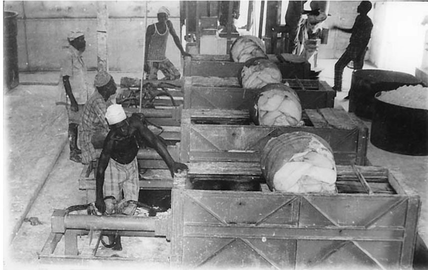
Figure 16 Commercial industrial gari production. Fermented cassava mash being dewatered in hydraulic presses. (Courtesy of the Federal Institute of Industrial Research, Oshodi, Lagos, Nigeria.)
