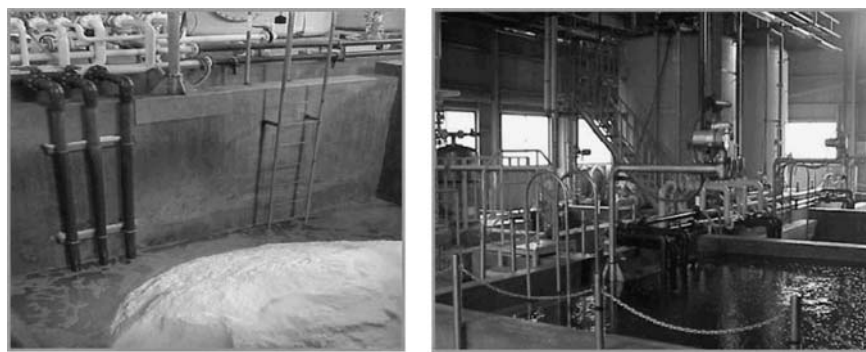
Figure 31 Brine-making facilities: left, solid salt; right, brine. (Courtesy of the Kikkoman Corporation.)
