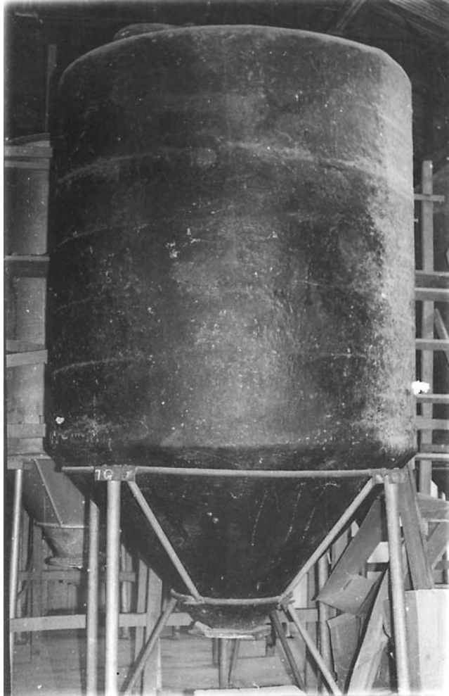
Figure 6 Storage of grain in a fiberglass silo. (Courtesy of the Federal Institute of Industrial Research, Oshodi, Lagos, Nigeria.)
