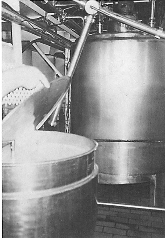
Figure 12 First stage of industrial-scale thermophilic starter preparation in a “prefermenter.”
