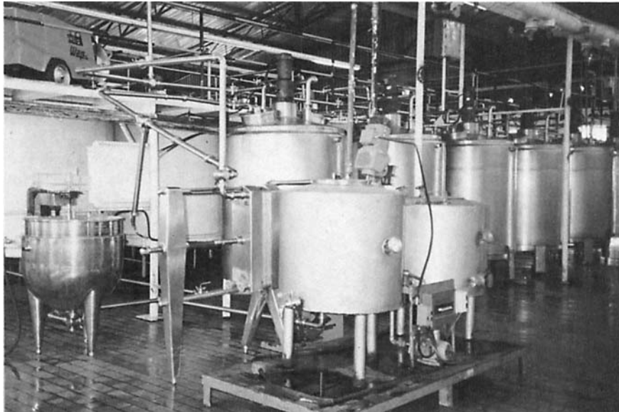
Figure 13 Second stage of industrial-scale preparation of thermophilic starter in 2000-L bioreactors. Small-scale prefermenters in foreground.
