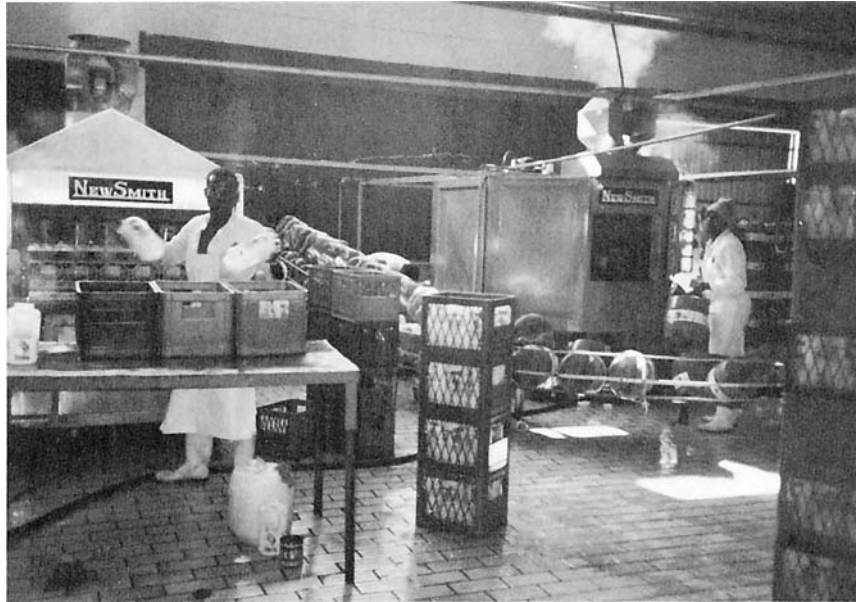
Figure 41 Washing of returnable 2- and 20-L plastic beer containers (South Africa). (Courtesy of the Sorghum Beer Unit of the Council for Scientific and Industrial Research, Pretoria.)
