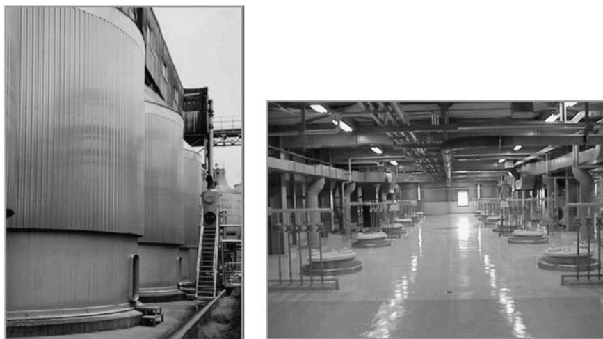
Figure 34 Modern fermentation tanks: left, outdoor large tanks used after 1970; right, indoor fermentation tanks made from glass fiber, used after 1975. (Courtesy of the Kikkoman Corporation.)
