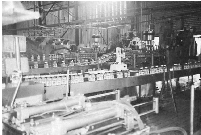
Figure 14 Packaging of the pasteurized mageu in 0.5- and 1-L cartons.
