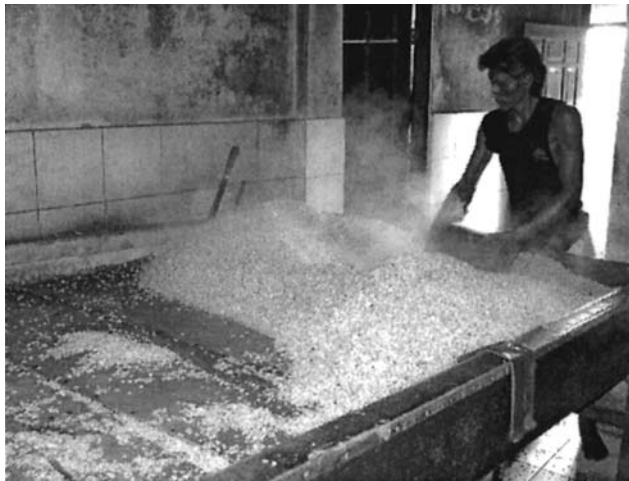
Figure 20 Draining and cooling tray.
