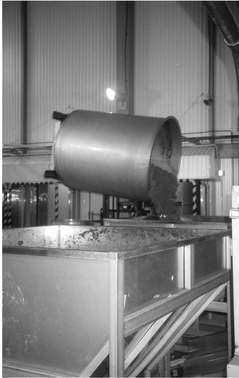
Figure 12 Turning a vat of miso (2 tons) transferred from the fermenting room with a fork-lift truck. (Courtesy of Sendai Miso Shoyu Co. Ltd.)
