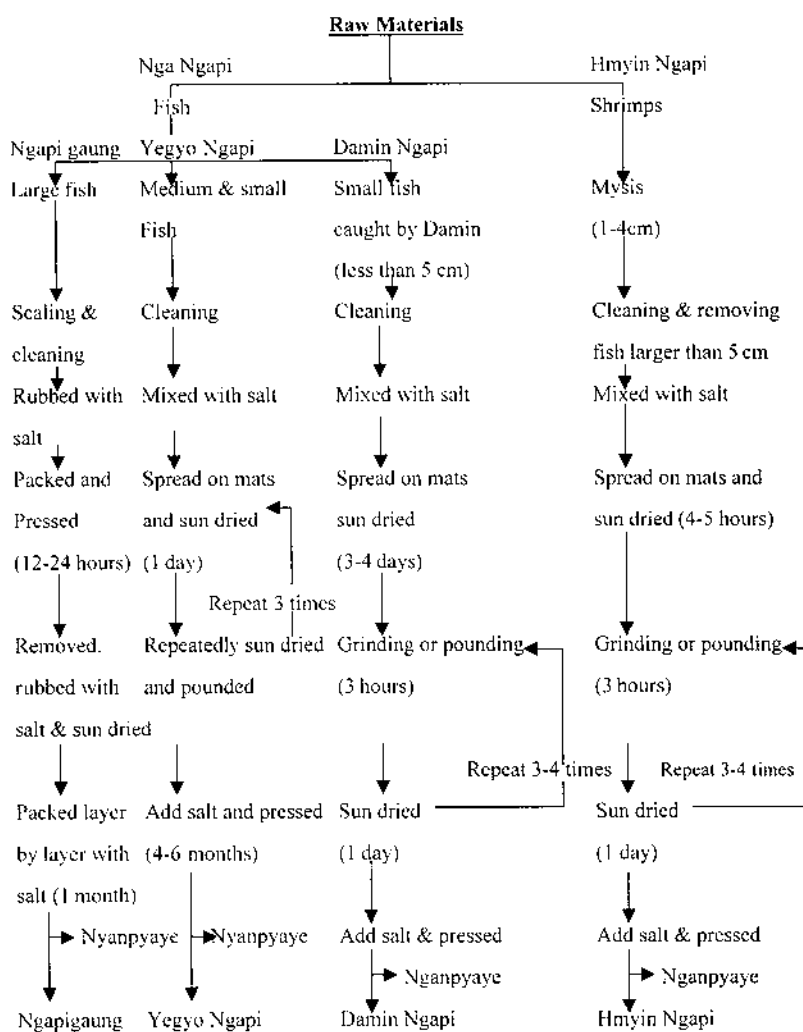
Figure 1 Process flowsheet for ngapi and nganpyaye.
