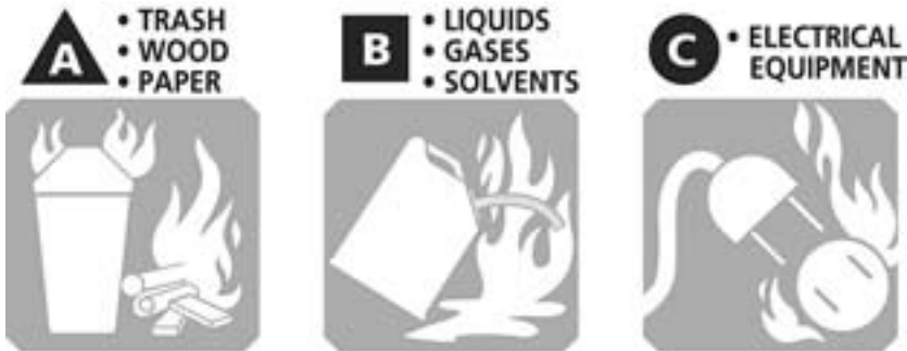
FIGURE 9.3 Standard labeling for fire extinguishers (Kidde Products)
