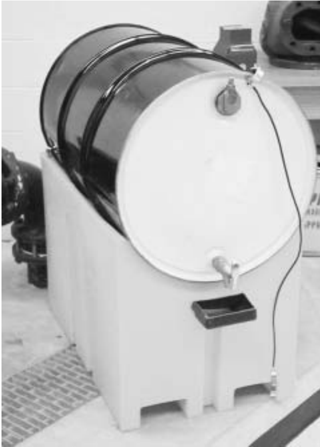
FIGURE 3.2 Typical flammable-liquids transferring arrangement
