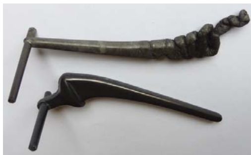
Figure 3.12 Jetting when the mould is filled from the thin end (the moulding is an experimental PEEK/CF hip prosthesis)
