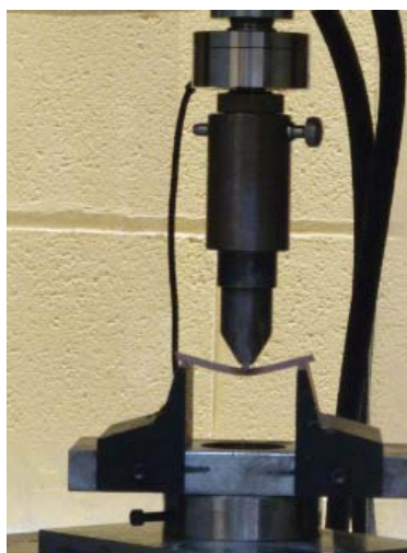
Figure 6.14 A specimen tested in 3-point bending
