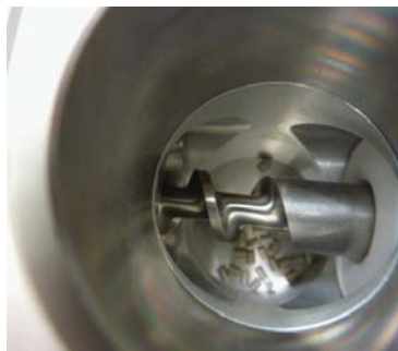
Figure 3.17 Hopper with an auger facility
