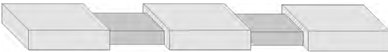
Figure 5. The very interesting experiment along a metallic waveguide with two barriers (undersized guide segments), i.e. with two evanescence regions [21]. See text.
