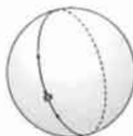
Fig. 10.4 A geodesic between two points on a sphere is an arc of the unique great circle on which they both lie
