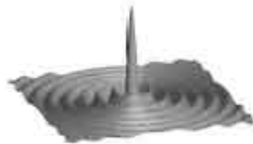
Fig. 8.3 A spherical wave. In general, the time-dependence need not be sinusoidal, but the amplitude always falls as 1/r as the waveform propagates out.
