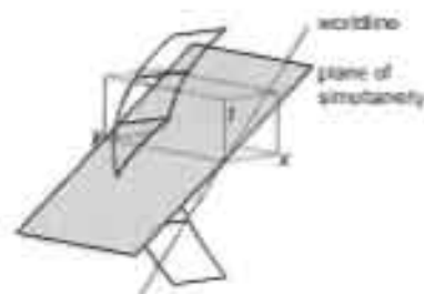
Fig. 6.8 Spacetime diagram showing the worldsheet of the accelerating stick shown in Fig. 6.7, and a plane of simultaneity for frame S' at t' = 0 (shaded). The stick is straight in the reference frame whose axes are indicated by the rectangular box ( x, y, t ); it is curved in the other reference frame because the plane of simultaneity intersects its worldsheet along a curve.
