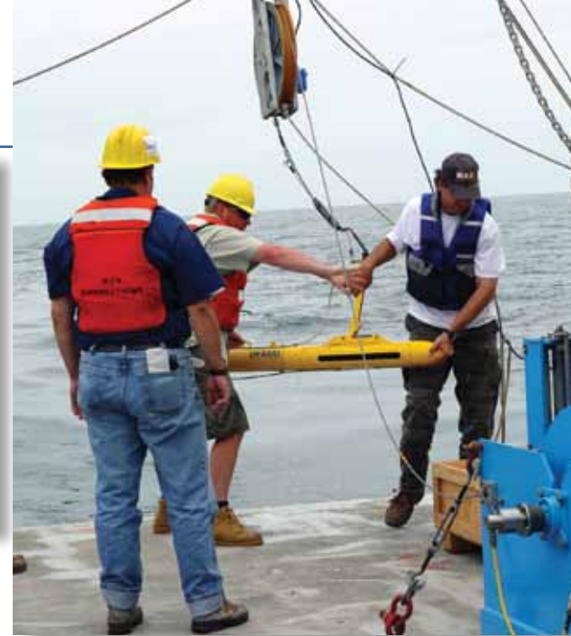
↑ The object above is used to "read" sound waves as it is towed below the vessel. You can see it being towed below. This is one type of sonar device.
