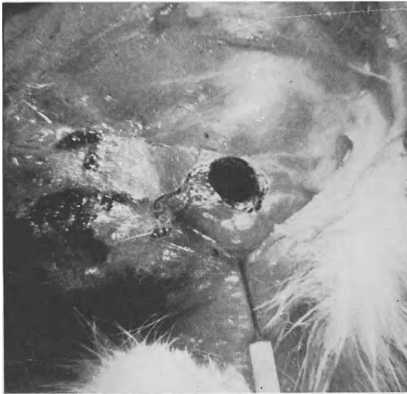
Fig. 15-3. Carbon dioxide laser impact on muscle tissue of guinea pig showing thermocouple to record temperature rise in tissue.
