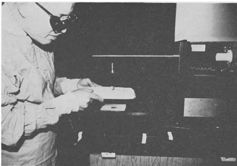
Fig. 2-7. Carbon dioxide laser, 20-watt output ( Perkin Elmer ) reducing a tooth to charred fragments.
