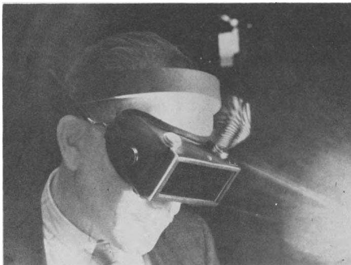
Fig. 20-6. Showing exposure of face on reflectance of laser beam from target area, temple area must fit tightly. Black-and-white copy of picture of laser impact color infrared Ektachrome (Eastman).
