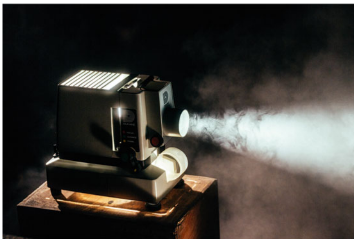
Fig. 3.27 You don't need "particleness" to describe why light travels in straight lines. The projector's aperture is very large compared to the wavelength of the light (approx. 0.05 m vs. 0.0000005 m). Given enough elbow room, waves propagate in straight lines due to interference effects.
