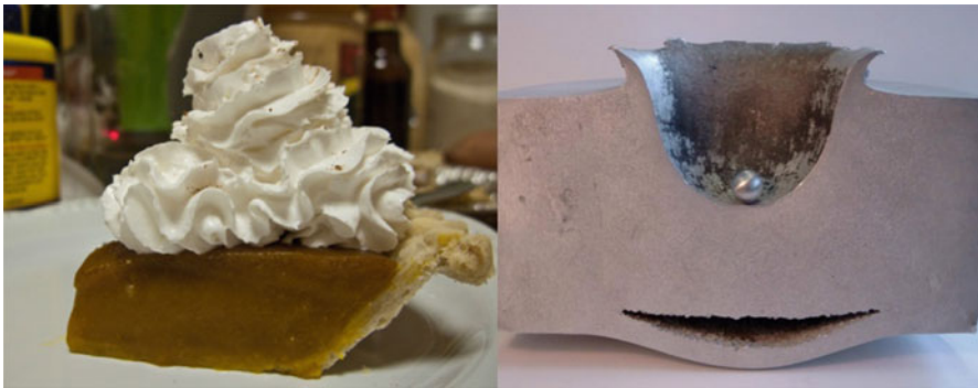
Fig. 3.51 Left: Whipped cream standing up like a solid at low speed. Right: Steel (recently) splashing like a liquid at high speed.
