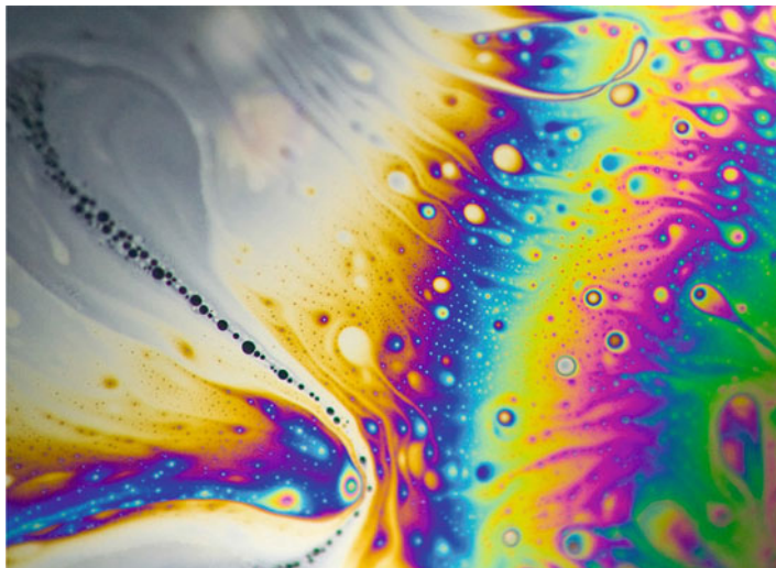
Fig. 3.29 Both the thickness of a soap bubble and the angle to your eye varies, so the colors that experience constructive interference (the colors you see) changes.
