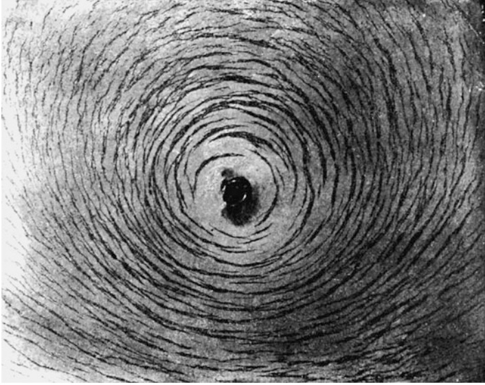
Fig. 3.45 “Magnetic fields curl around current”. Iron filings have the convenient property that they tend to line up with magnetic fields, so a current-carrying wire going through a piece of paper covered with iron filings will arrange them thusly.
