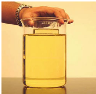
Fig. 3.16 When light moves between materials with different indexes of refraction it can either pass through the boundary or reflect. The smaller the difference in indexes, the less light will reflect. In this picture both glass beakers and the fluid they contain all have the same index, so light is free to pass from one substance to the next without any reflection, making the inner beaker invisible.
