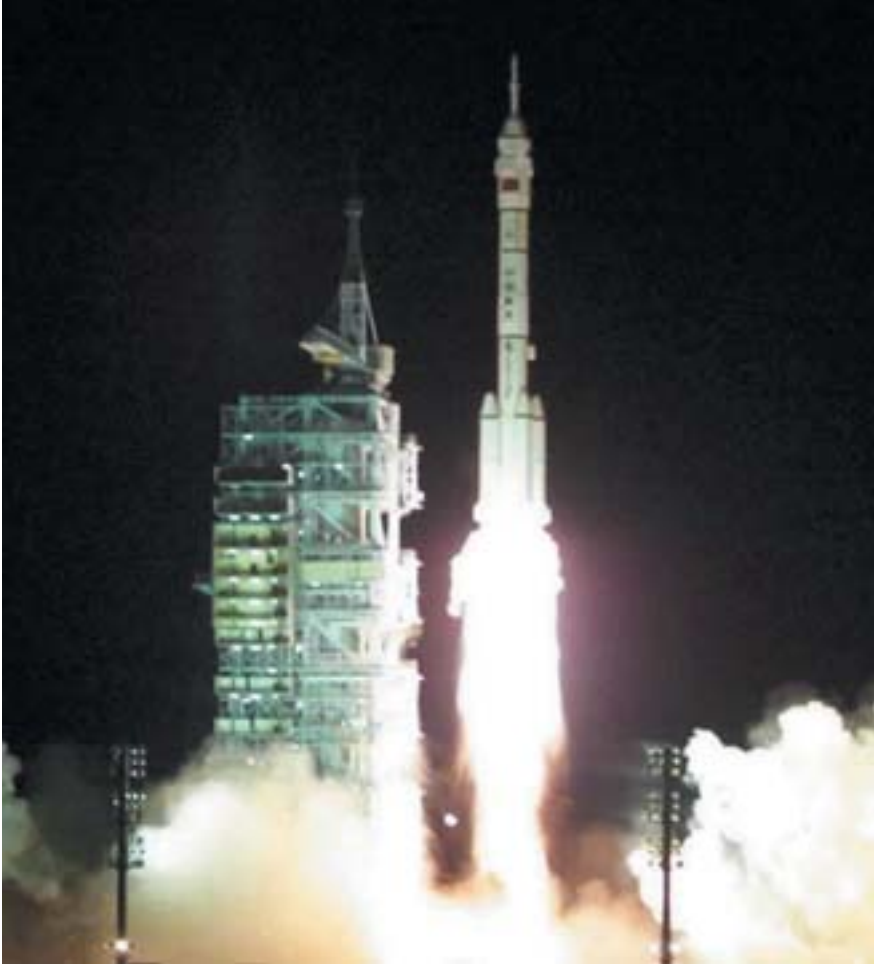
UNMANNED TEST FLIGHT of Shenzhou 2 began with a night launch on January 10, 2001. The two-stage Chang Zheng 2F rocket gets added thrust from four strap-on boosters at its base.
